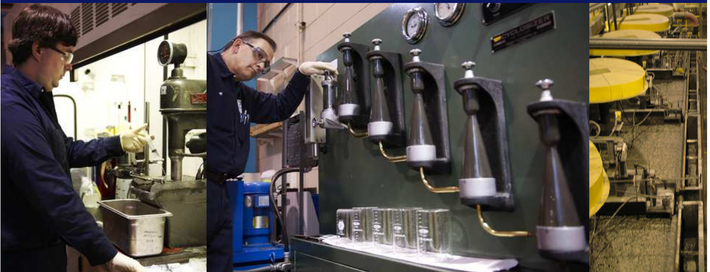
Technicians at XPS performing flotation and cyclosizing testwork (above left and centre).
